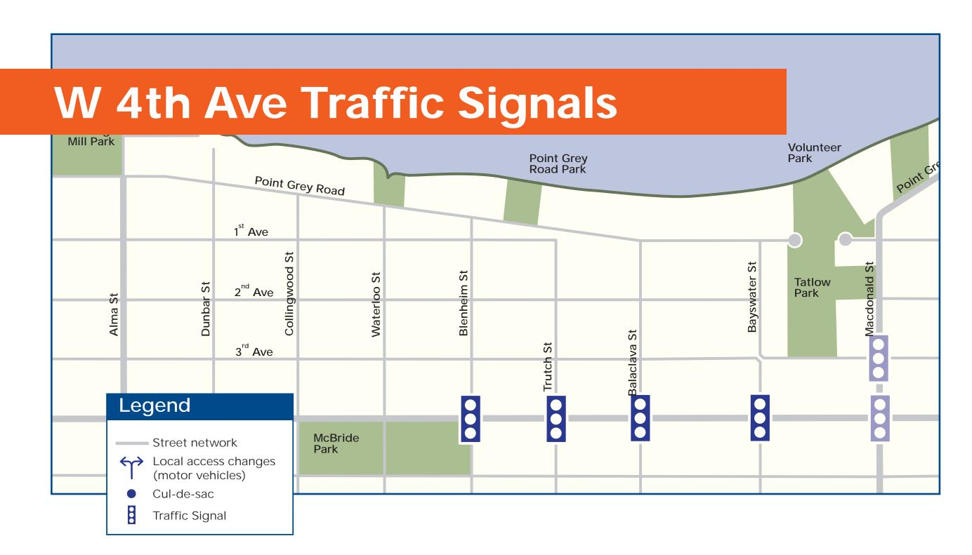
Prior to 2014, the traffic signals on 4<sup>th</sup> Ave at Blenheim St, Trutch St, Balaclava St and Bayswater St stayed green for traffic travelling on 4<sup>th</sup> Ave unless a person walking or cycling pushed a button to change the light.
